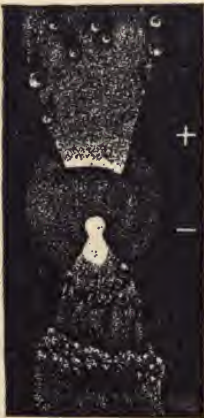
FIG. 387. — The Electric Arc Produced by a Direct Current.
